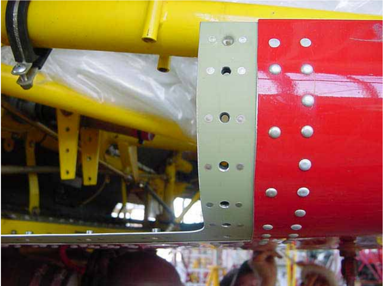
Image #5 Close up of Access panel doubler installed.
