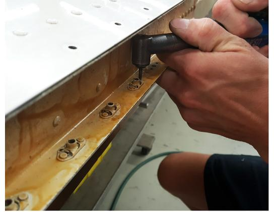
Grind or drill off rivet tails
