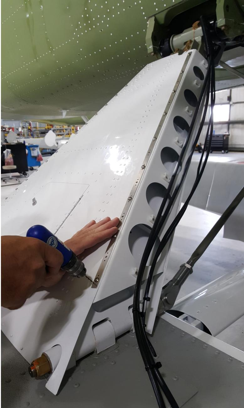
16. Position and secure 1008970 drill template as shown and drill out existing nutplates using a #40 drill bit
