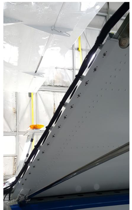
22. Reinstall pulleys and rig water rudder retract and steering cables per Wipaire Service Manual PN 1005723
