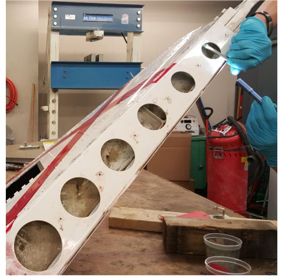
20. Apply PPG Aerospace PR-1422 B-2 sealer to (1) 1008969 nutplate strip assembly and (1) 1008967 nutplate strip assembly and install each one where shown
