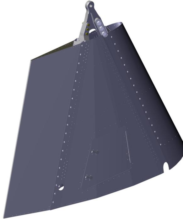
24. Reinstall pylon fairing assembly using previously installed hardware
