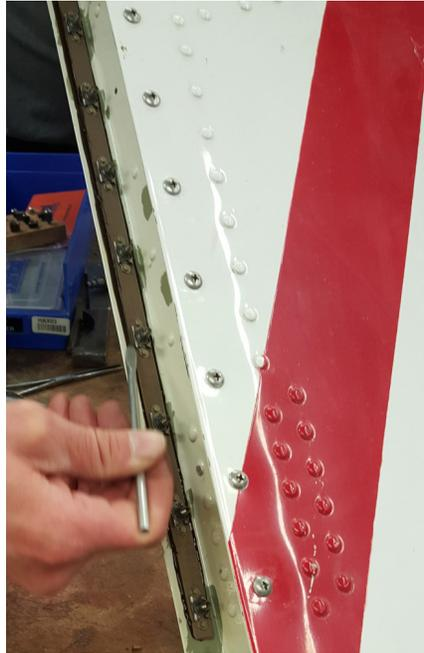
12. Apply a 1 inch piece of 9903-13-36 barrier tape to (5) MS21060L08 nutplates and backdrill through tape in the locations shown
