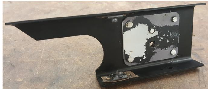
14. Position lower pulley bracket and nutplates inside of drag strut channel with clecos and install through drag strut channel with rivets MS20426AD3-4.5
