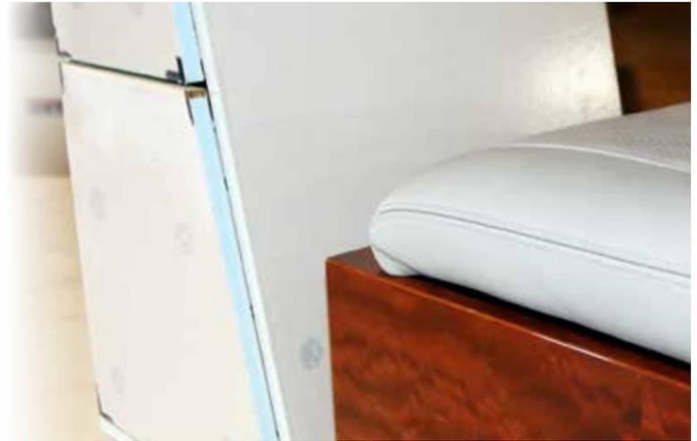
A completed cabinet next to a two drawer unit that has not received its veneer finish.
