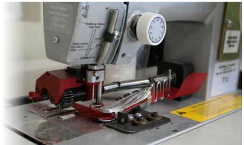
A special upholstery machine designed for binding carpet edges for a neat finish.
