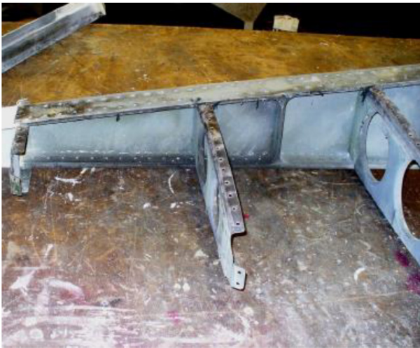
Pylon before repair...
