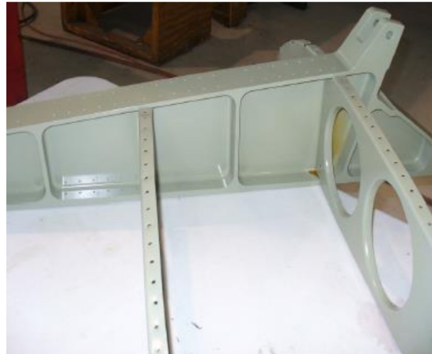
Pylon Fully Repaired
