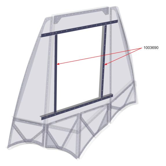
3. Inspect 1006080 Bulkhead Main Panel for cracking. If cracking is found, contact Wipaire Customer Service to receive additional instruction for repair. If no cracking is found, proceed to the next step
