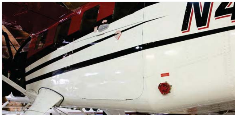
The Single Point Fueling adaptor is located just aft of the left-hand aft door for easy access by refueling personnel.
