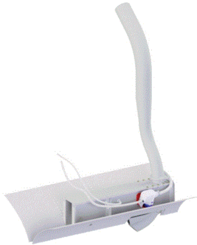
Bilge Pump On Scoop Tunnel
