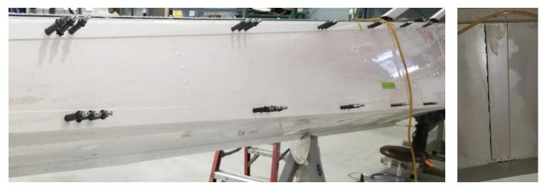
6. Rivet stiffeners to gunwall and chine, as shown below.
