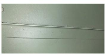
Condition 3 - Corrosion visible under stiffener, and corrosion has spread into the skins.
