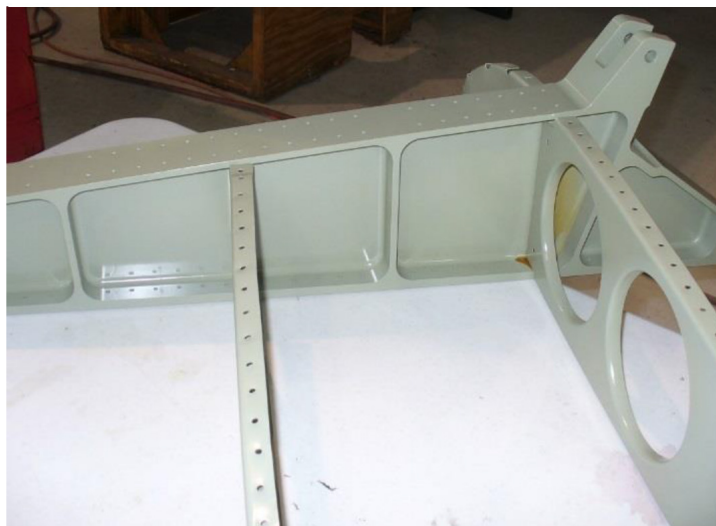
Pylon fully repaired
