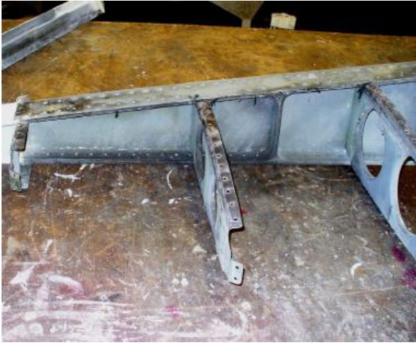
Pylon before repair...
