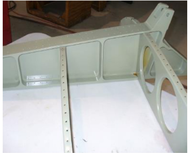
Pylon Fully Repaired
