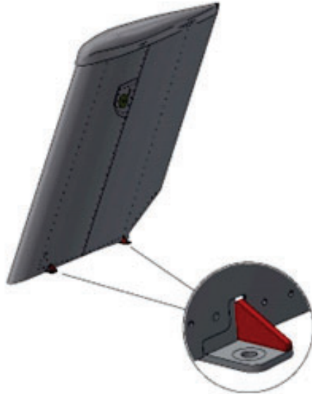
Figure 8 Finlet Mount Weldment Gussets
