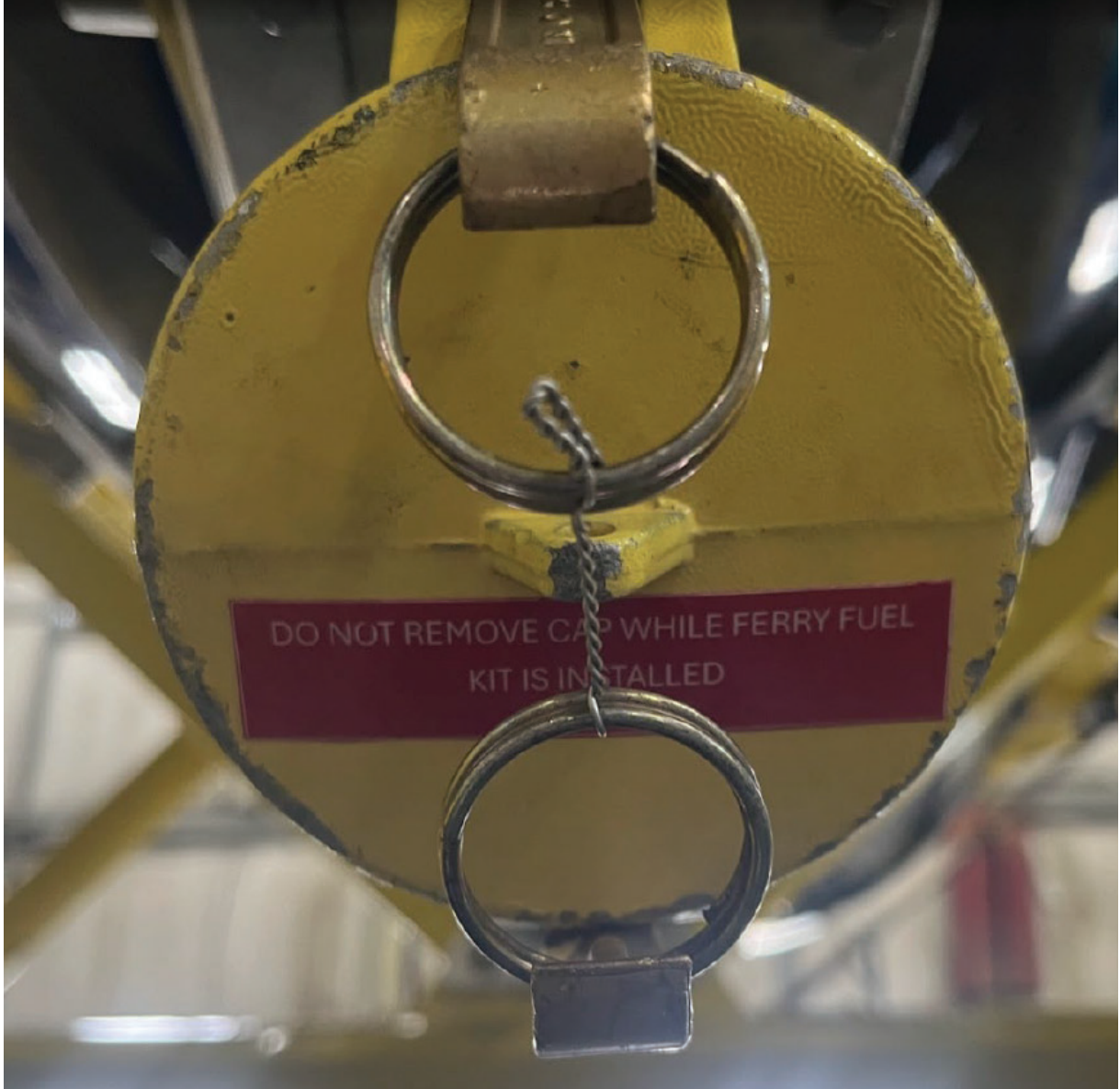
Figure 7 - Ground Fill Cap
