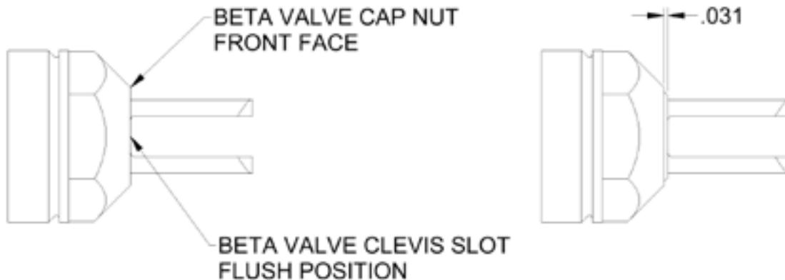
FIGURE 2, ACCEPTABLE RANGE OF BETA VALVE ADJUSTMENT
