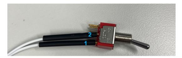
5. Near the Master Caution or Master Warn light, locate a space to install the supplied momentary switch and placards. Ensure ample space to install both switch and placards in proper orientation. Drill a 1/4-inch hole and install the switch with the provided hardware.
