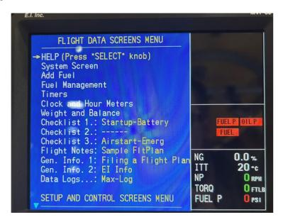
2. Scroll down and select "USB and Data Recording." If prompted to enter a password, enter either 00100 or 00200. Press "EXIT" when password is entered.
