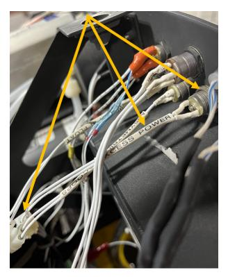
6. Properly stow the opposite wire lead. Place the nylon hole plug (Item 6) in place of the light assembly. Remove the ENGINE POWER placard and replace it with the new placards (Item 7, Item 8).
