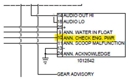
3. Using a D-Sub pin removal tool, remove the Check Engine Power pin from the D-Sub connector. Once removed, properly cap and stow the wire. If a pin removal tool is not available, cut the wire and properly cap and stow both ends.
