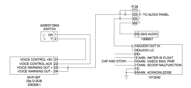
1. Locate and remove the MVP-50T 25 pin D-sub connector. For ease of access, it may be beneficial to remove the MVP-50T display from the panel by removing the four Philips head screws that secure the display to the panel.
