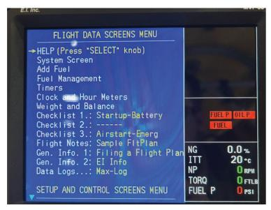
3. Scroll down and select "System Configurations Screens." Then select the "USB and Data Recording" menu. If prompted to enter a password, enter either 00100, 00200, or the aircraft serial number. Press "EXIT" when password is entered.
