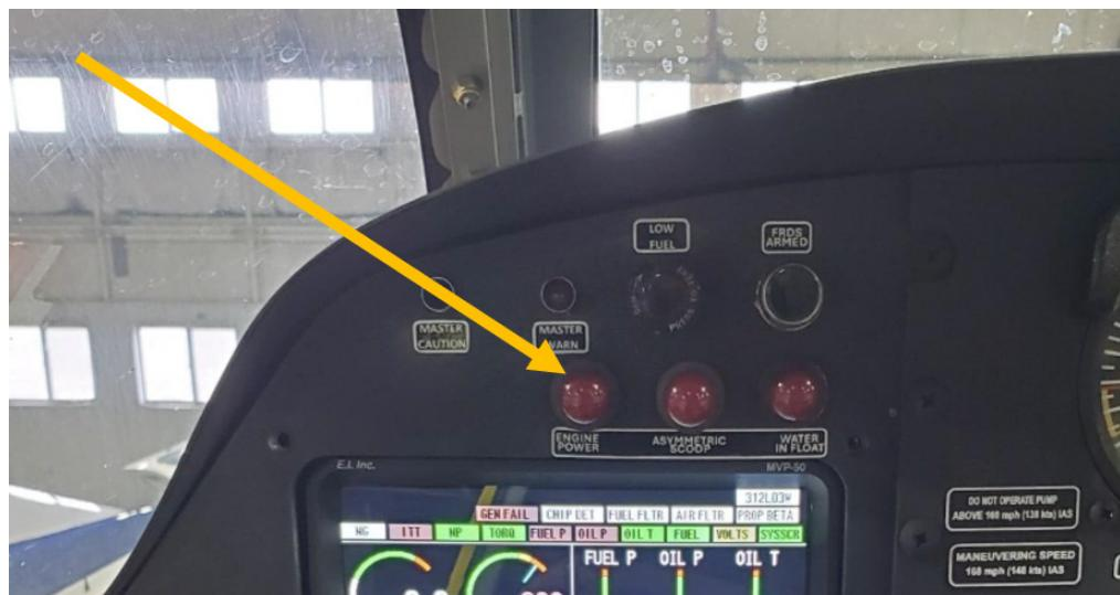
5. From the backside of the light, undo the connector on the wire tail labeled "EXCESS POWER". Remove the nut on the backside of the light and remove the light assembly with the wire tail. \*\*Optional, see step 8.
